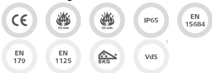
CE tested | EN 1634: 30 minutes | EN 1634: 90 minutes | IP65 rating | EN 15684 | Suitable for locks as per EN 179/1125 (when using the FAP anti-panic function)
