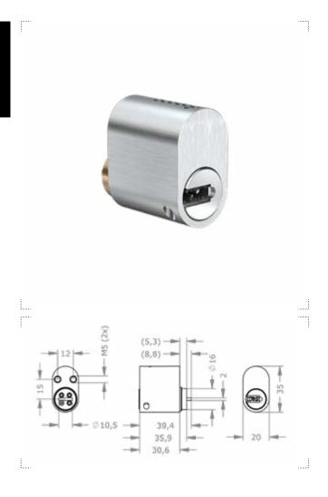
**FUNCTION** Can be locked with key Reversible key **USAGE** Door exterior, connecting doors, entrance doors, apartment entrance, metal frame door, security **ASSEMBLY** For Scandinavian mortise locks **SECURITY** Pin rows: 6 Active pins: Drilling protection: Pulling protection: Picking protection: Security card: **STANDARDS** EN 1303:2015 160B0C6B Fire resistance 90 minutes INCLUDED COMPONENTS Cylinder lock
