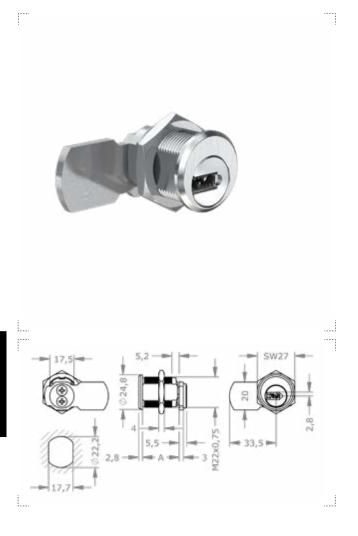
**FUNCTION** Can be locked with key Reversible key Locks with cam at the rear side **USAGE** Glas cabinets, mailboxes, key boxes, technical distribution cabinets **ASSEMBLY** Hole pattern d > 22 mm Flattened on the side Fixed on the back by a flat nut **SECURITY** Pin rows: 6 Active pins: Passive pins: 10 Security card: **STANDARDS INCLUDED COMPONENTS** Cylinder lock Cam H7233 mounted Hexagon nut
