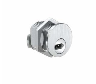
**FUNCTION** Can be locked with key Reversible key Locks with cam at the rear side **USAGE** Glas cabinets, mailboxes, key boxes, technical distribution cabinets **ASSEMBLY** Hole pattern d > 30 mm Flattened on the side Fixed on the back by a flat nut **SECURITY** Pin rows: Active pins: 6 Passive pins: 10 Security card: **STANDARDS INCLUDED COMPONENTS** Cylinder lock Cam H7233 mounted Hexagon nut
